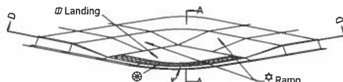
BLENDED TRANSITION THRU CURB RADIUS (ALT. TYPE 3)
